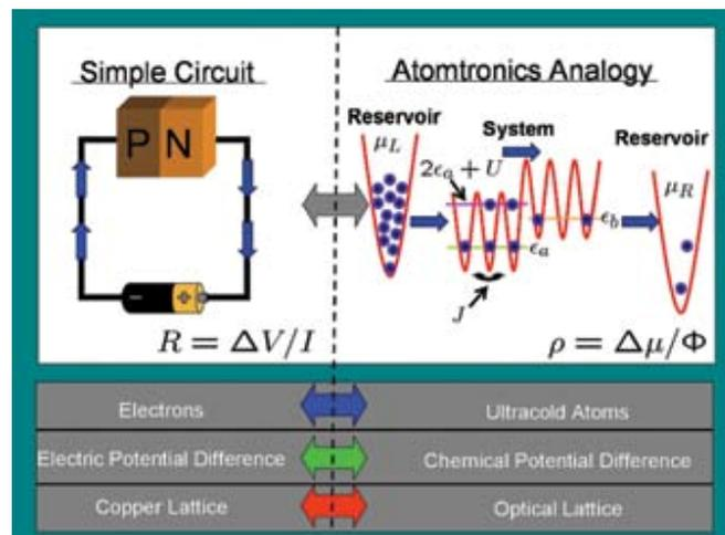
**Fig. 2: Atomtronic analogy to diode circuit**
