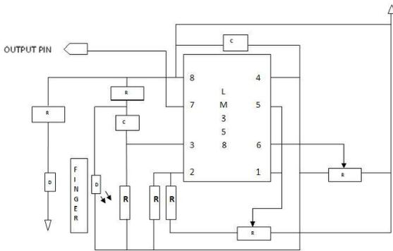
**Fig. 3.** Pulse Sensor Circuit
