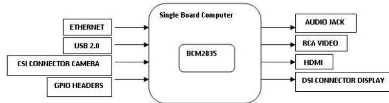
**Fig. 3.** Single board computer (Raspberry pi)
