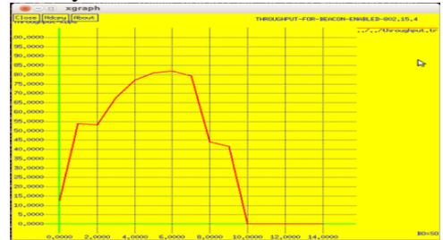
Fig. 12. Throughput vs BO=SO in Star Topology in Beacon- Enabled Mode
